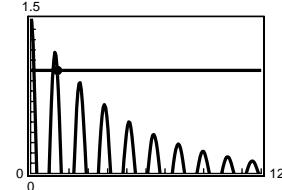
The displacement does not exceed one inch from equilibrium after  $t = 1.96$  seconds.
